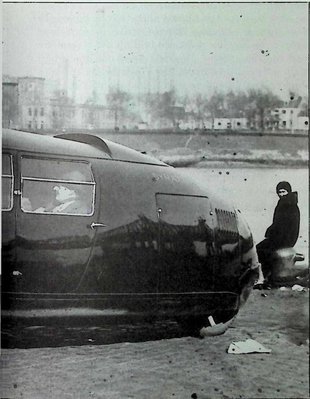
Fuller's Dymaxion Vehicle. The rear wheel steered the streamlined, tear-shaped vehicle, acting much like the rudder of a ship.
