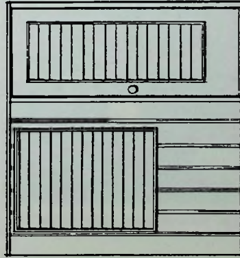
2621 or 3921 (If door is desired on left side, please specify.) 3'1" x 4'2 3/8" aluminum-glass jalousie window with screen, and swing-out jalousie door, also with screen panel.
