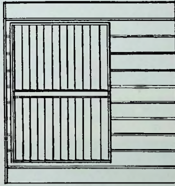
2622 or 3922 Two wide, one high aluminum-glass jalousie window units with screen panels.
